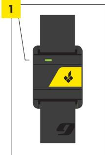
**1** turn the heart rate monitor on; the light must be green connecting the monitor with the bike is automatically
