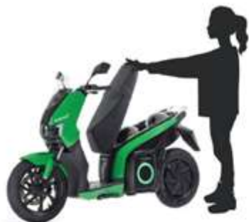
Open the seat with the APP, with the key, or pressing both brake levers
