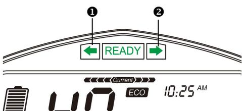
An arrow on the upper speedometer flashes green in the same direction as selected by the steering lamp switch. This remains flashing until the steering lamp request has been canceled.
