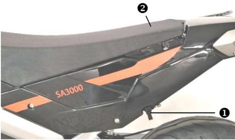
The seat/helmet lock is located at the rear left side of the motorcycle.
