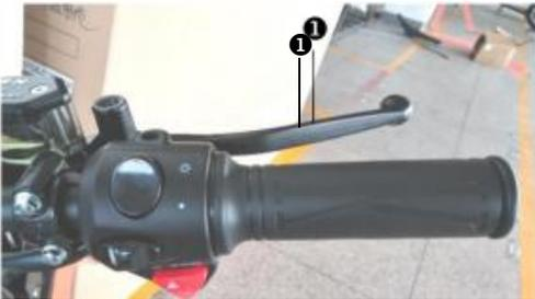
The front brake handle ❶ is fitted on the right side of the handlebar.
