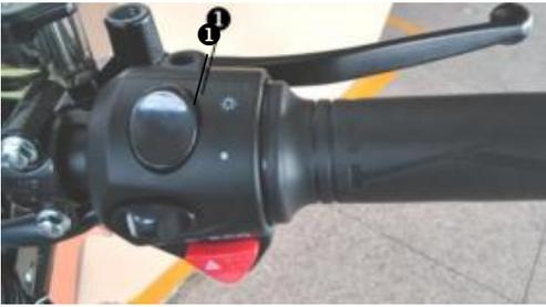
Flip the switch upward to ☀, open the Headlight.
