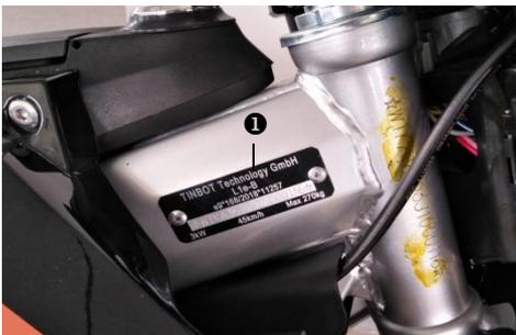
The nameplate ❶ is mounted on the chassis at the front right.
