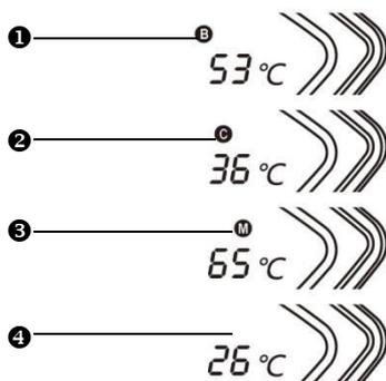
The system can display four temperatures, with "B" above the temperature display value indicating current battery temperature, "C" indicating current controller temperature, "M" indicating current motor temperature and no label indicating current external temperature.
