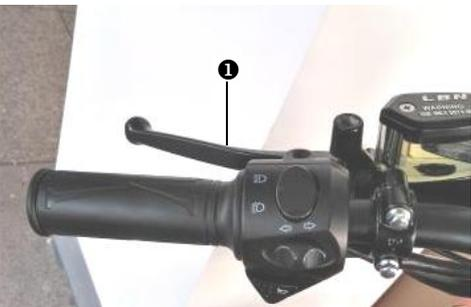
The rear brake lever ❶ is fitted on the left side of the handlebar.
