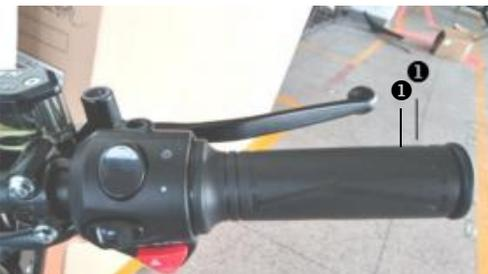
The throttle grip ❶ is fitted on the right side of the handlebar.
