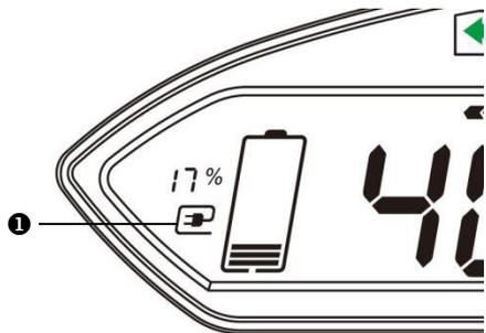
This charging indicator symbol ① display when the battery is charging.
