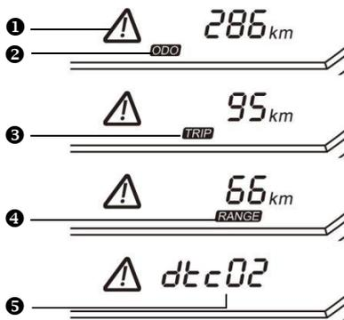
When the error code indicator <sup>①</sup> turns on, it indicates a fault in the motorcycle. The error code is displayed in the odometer.
