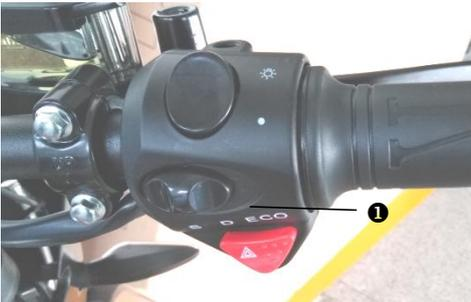
The driving mode switch ❶ is on the right handle switch.
