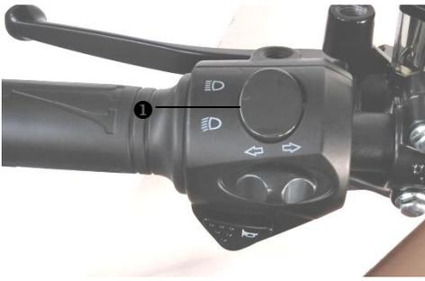
The headlight high/low beam ❶ switch is on the left handle switch.
